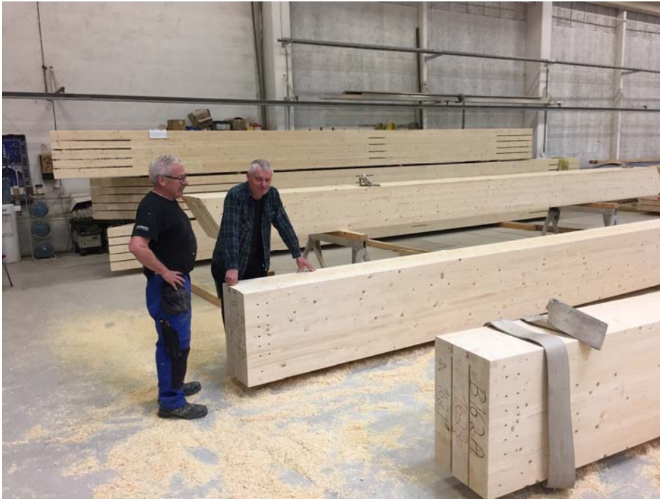
Production of truss diagonals
