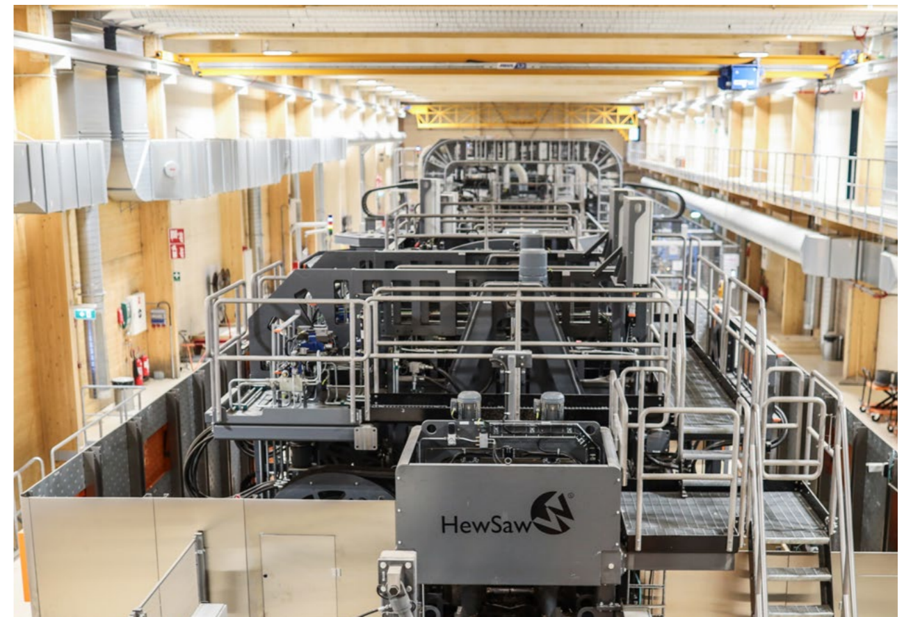
When Moelven Edanesågen AB invested in a new sawing line, the associated building was constructed using a load-bearing structure made of glued laminated timber and wall/floor elements of solid wood, a total 674 m 3 . These materials store biogenic carbon equivalent to around 470 tonnes of CO 2 . For context, the World Population Review ( www.worldpopulationreview.com ) has calculated that average CO 2 emissions per capita in Norway and Sweden in 2023 were 7.8 tonnes and 3.4 tonnes respectively.
