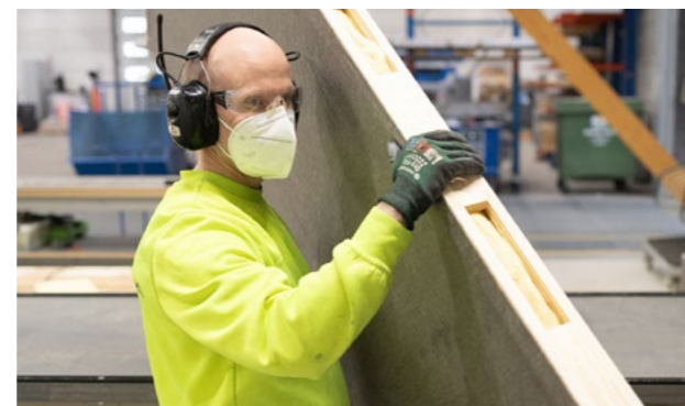
Loop Wall, which is part of Moelven Modus AS's standard range, is a patented prefabricated wall system designed for reuse. The wall has a wooden core and is developed and manufactured at Moelven's factory in Jessheim. Loop Wall is easy to handle and quick to assemble and reassemble, making it ideal for office buildings.
