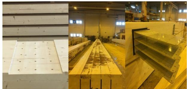
**Figure 14:** CNC processing / Block gluing / Installation of steel plates
